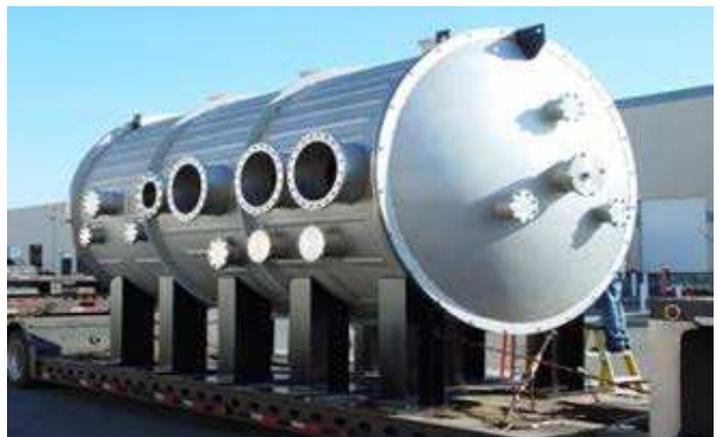
**Vacuum Vessel for use in Space Simulation Courtesy of GNB**
