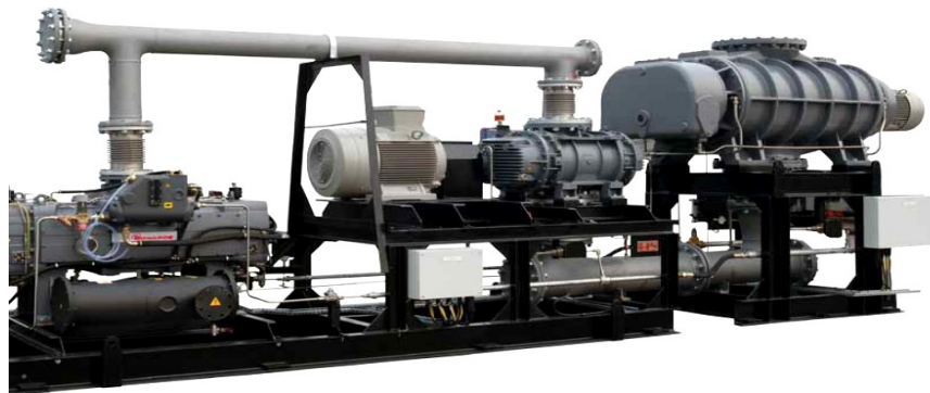
Fig. 7. Edwards mechanical pumping system with pumping speed 1,000,000 m 3 /hour [6].
